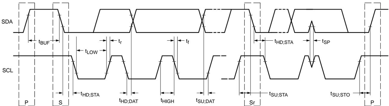
Figure 15. Definition of Timing on the I<sup>2</sup>C Bus
