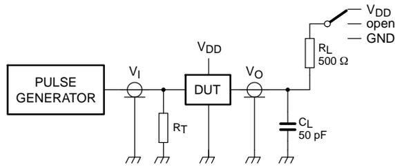
$R_L$  = load resistor.
