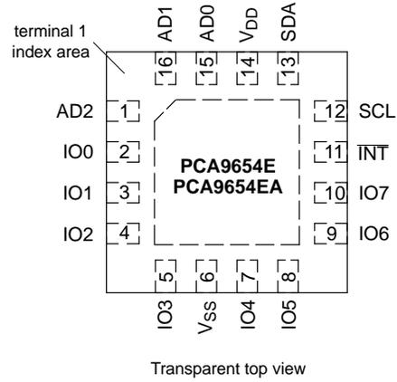
Figure 4. WQFN16 / QFN16
