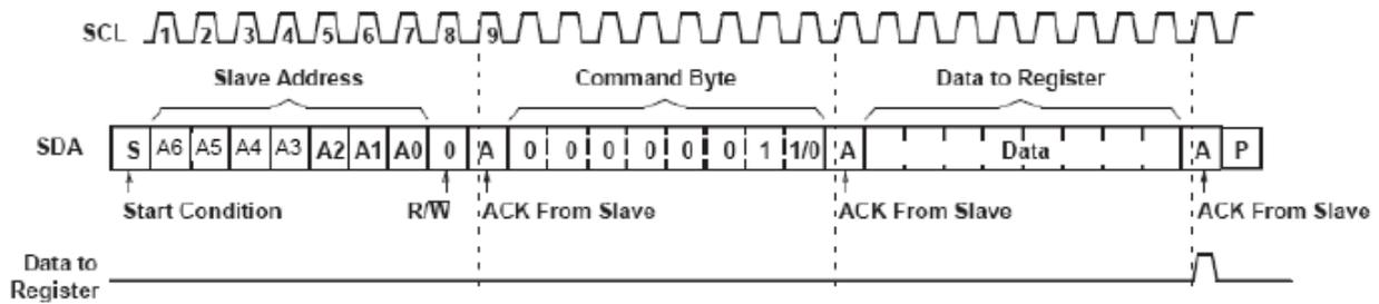
Figure 7. Write to Configuration or Polarity Inversion Register
