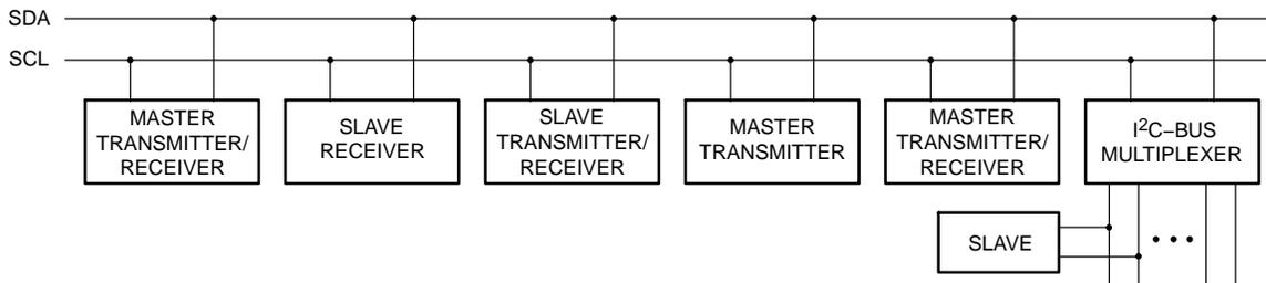
Figure 13. System Configuration
